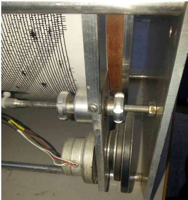
*The rotation-motor assemblage of the Landsnet seismograph. It offered three different speeds of rotation. The most used time resolution was 90 mm per minute.*
