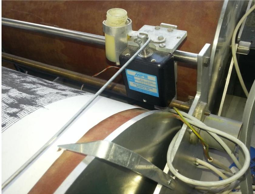
*The pen-motor and translation-motor assemblies of the Landsnet seismograph. The pen was made at the SI from a drawing pen tip attached to a syringe pipe. A special recording ink was used, available in different colors, black, red, green and blue.*
