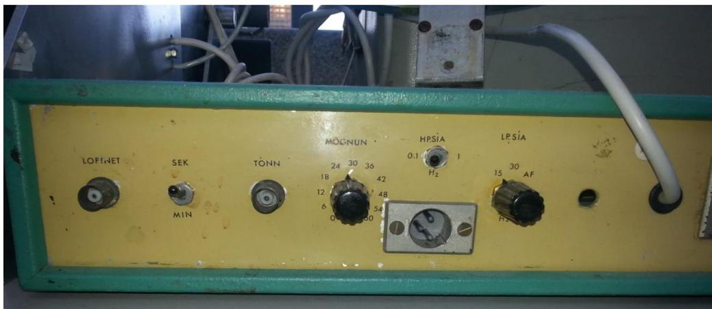
*The front of the electronics box: Input for the time signal antenna, seconds filter, tone input for FM modulated signals from a signal receiver, amplifier 0-60 dB, HP-filter, input for geophone signal, LP-filter, 220 VAC power cord, 12 VDC power input.*
